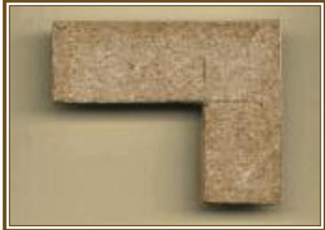
*The mitre corner is overcut onto the false corner to ensure a clean corner*
